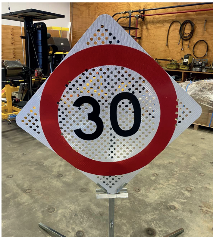
WSP Research is assessing holey temporary traffic signs to improve their resilience in strong winds. The theory being tested is that wind will pass through the holes – meaning the signs will experience less wind load and be less likely to blow over. Apart from school patrol lollipops, perforated signs aren't used in New Zealand. Photo: WSP Research.
